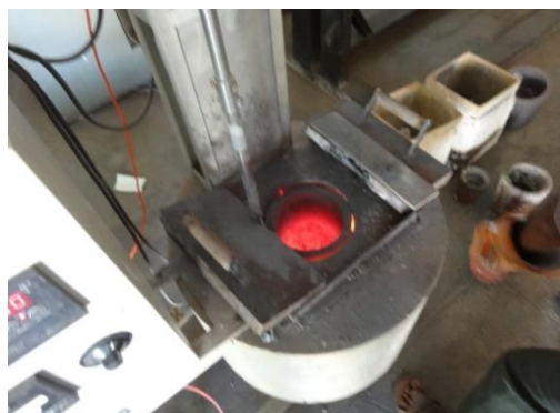
Figure 1. Experimental setup for making stir cast.
