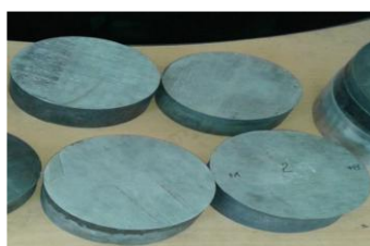
Figure 2. Al 2014-10wt%SiC composite after extruded it to 1:4 ratios.
