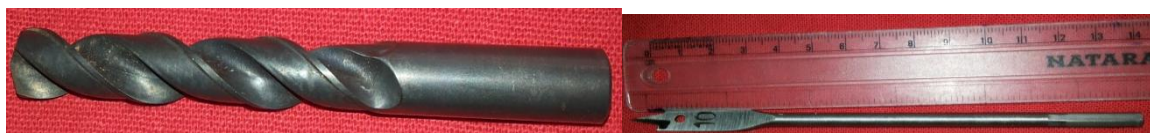
Figure 4. Drill bits of Ø 10 mm (a) Twist drill (b) Spade drill
