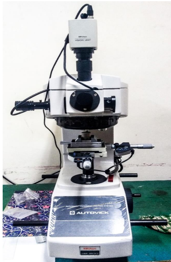
Figure 2. Hardness testing of prepared composites
