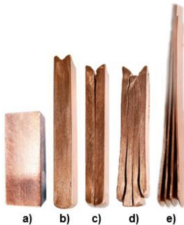
Figure 3. Processing copper by MDE+R: a) initial billet; b)...d) 2 nd , 3 rd , and 4 th MDE pass; e) final rolling.
