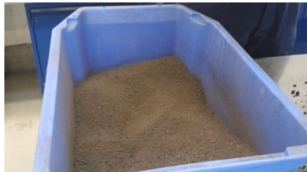
Figure 6. Sludge prepared for pelleting.
