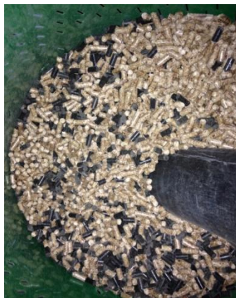
Figure 11. Mixture of sawdust and sludge pellets prepared for incineration.
