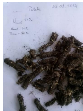
Figure 4. Sample 2. Pellets from sludge (30% sludge – 70% straw).
