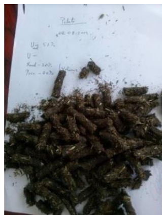
Figure 3. Sample 1. Pellets from sludge (20% sludge – 80% straw).
