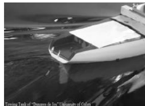
Figure 5. Hydrodynamic flow spectra, v=1 m/s (full scale 6.2 Kn).
