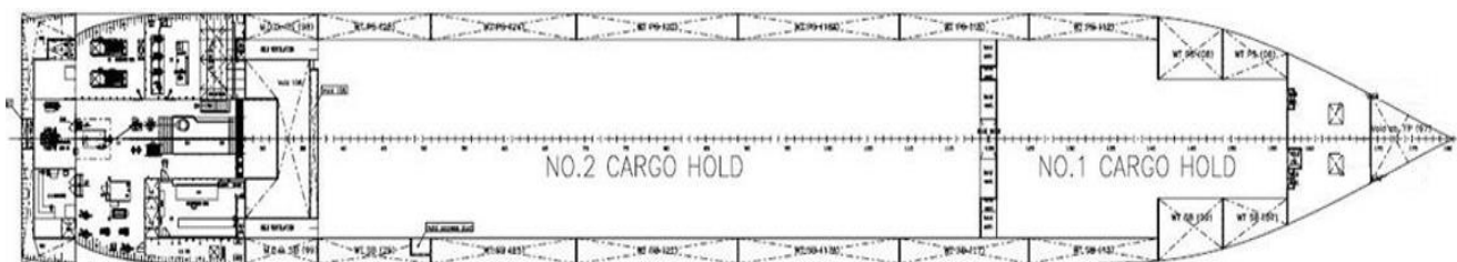
Figure 1. Illustration ship's cargo holds and ballast tanks arrangement.
