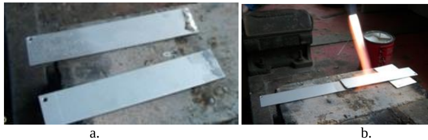
Figure 3. Characteristics of brazing technology parameters a. Filler material deposition on both sides of the base material, b. the use of a neutral oxyacetylene flame.
