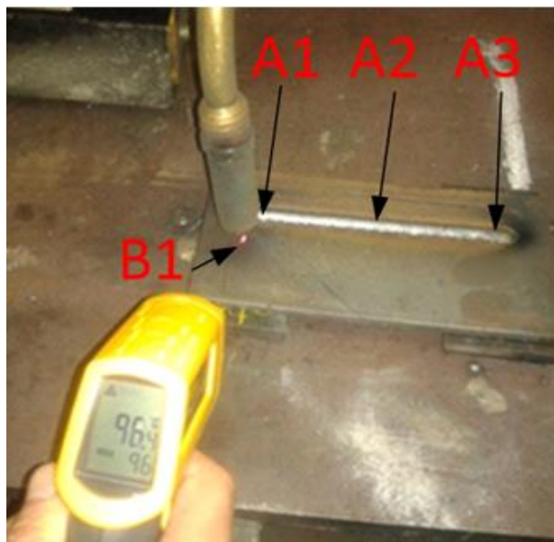
Figure 3. Temperature measurement A1 - the beginning of the seam previously deposited, A2 - the middle area of the seam previously deposited, A3 - the ending area of the seam previously deposited, B1 - the beginning area of the following seam.
