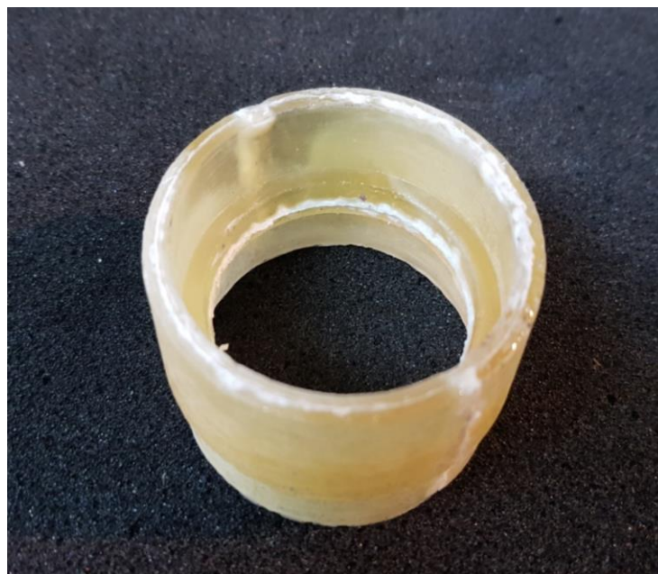
Figure 3. The worm bushing is cast in PDCPD class material with visible sockets under the bearing.
