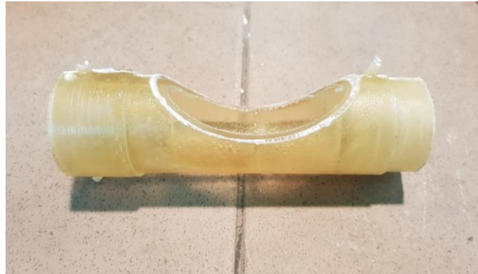
Figure 2. Worm sleeve casted in PDCPD class material.
