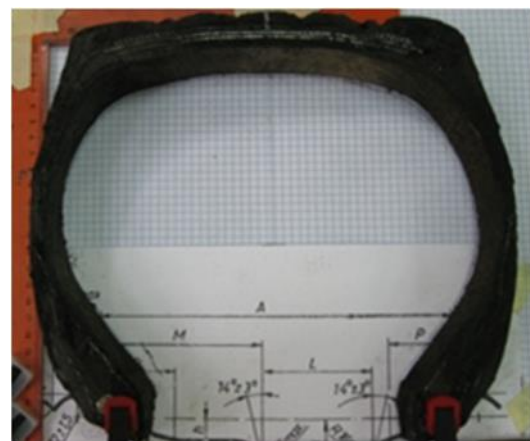
Figure 2. Section of 11R22.5 truck tyre used for measuring contour coordinates.
