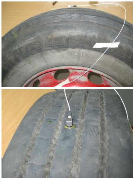
Figure 6. The tyre instrumented with a piezoelectric accelerometer.
