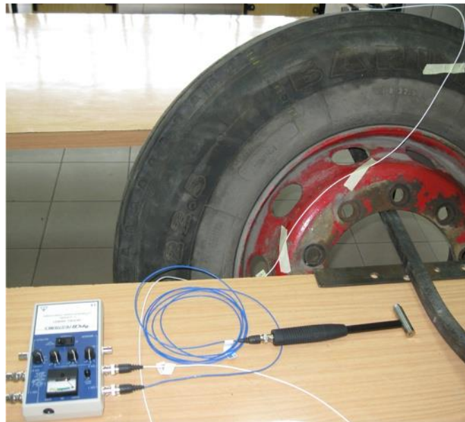
Figure 7. The measuring system for investigation of tyre modal behaviour using the impact hammer method.
