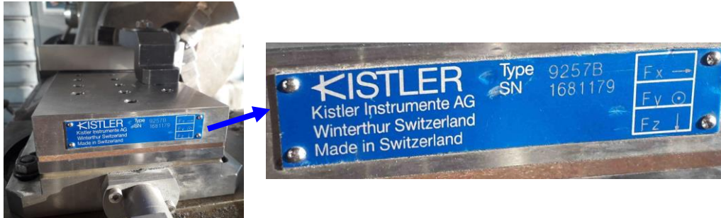
Figure 2. Dynamometer position on the machine tool.
