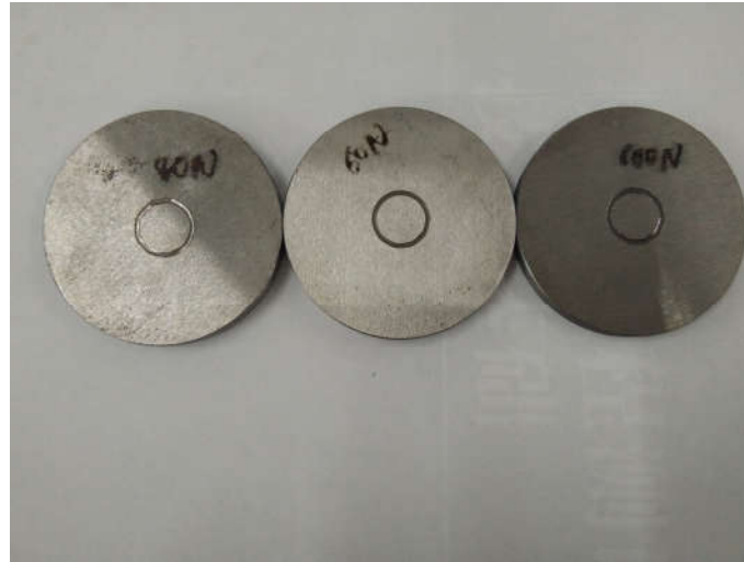
Figure 13. Wear scars of different test pieces.
