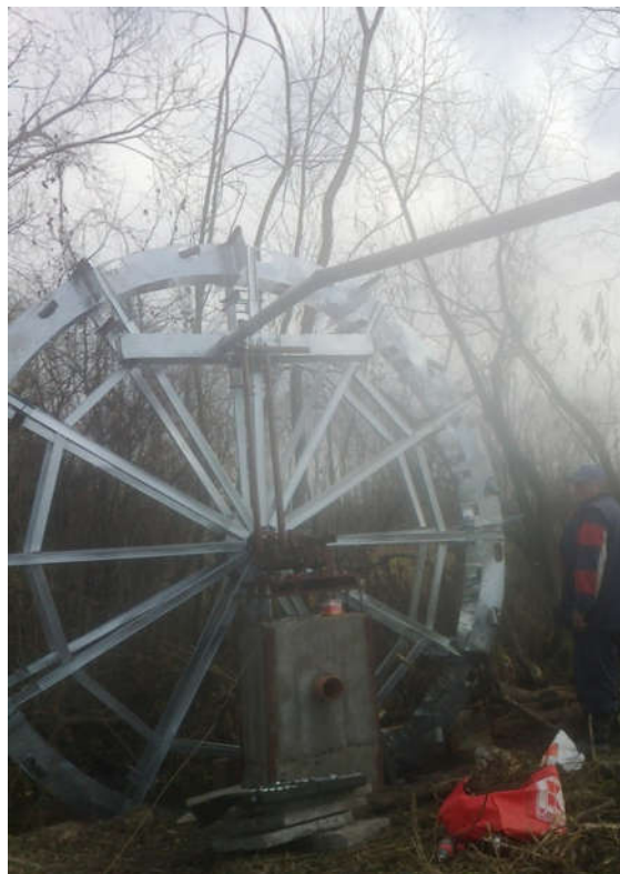
Figure 16. Undershot water wheel used for irrigation of dry lands.
