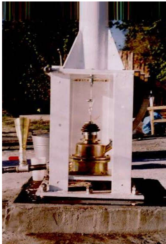
Figure 11. Diaphragm pump used to pump water.
