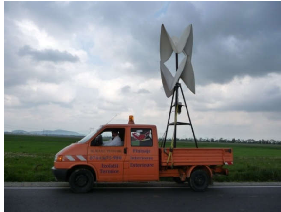
Figure 7. The experimental tests of two rotors helical type on vertical axis wind turbine.
