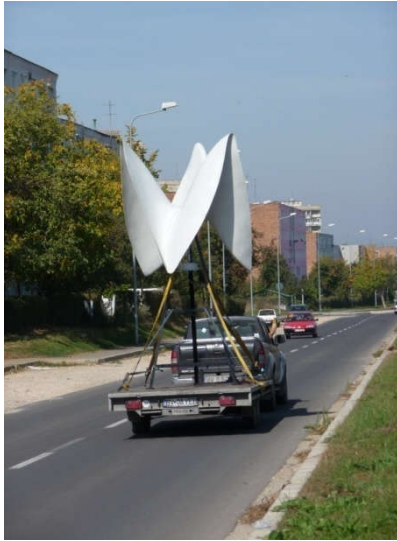
Figure 5. Wind turbine with vertical axis helical type mounted on a car during experimental tests.
