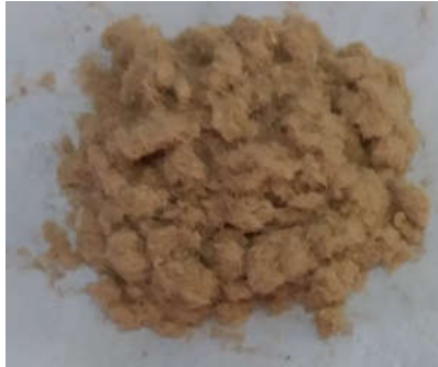
Figure 3. Wood fibres composed of 80% resinous wood and 20% beech wood, used in the present research as filler for the new composites.
