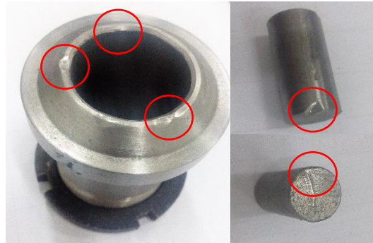
Figure 2. Impact damage on the sabot separator and the projectile
