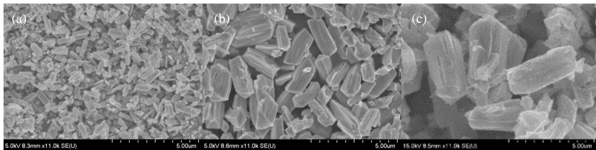
Figure 1. FESEM images of samples: (a) NiO 50 °C(60 min), (b) NiO 75 °C(60 min), and (c) NiO 100 °C(60 min) at constant co-precipitation dwelling time of 60 min
