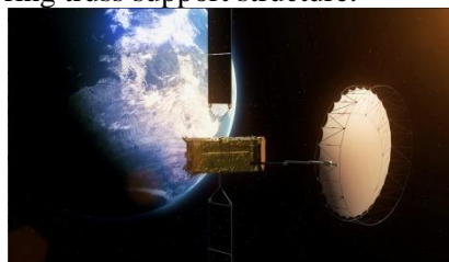
Figure 1. Truss antenna reflector.
