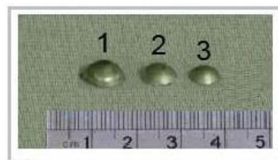
Figure 4. Plugs created due to different firing velocity.
