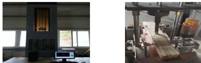
Figure 5. Experimental setup of low-velocity impact test.
