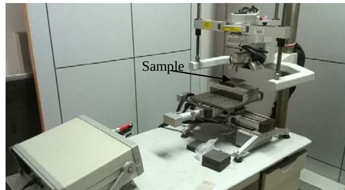
Figure 3. Xstress 3000 type X-ray stress analyzer
