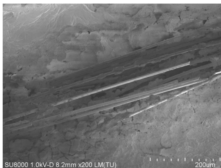
Figure. 1 SEM observation showing the cross-section of the Sic fiber/ \text{ZrO}_2 composite TBC layer
