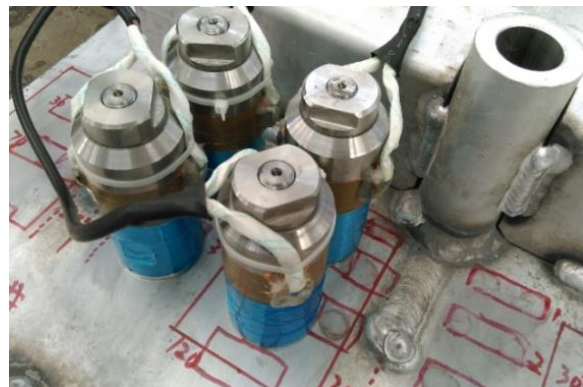
Figure 7. Site layout of the ultrasonic transducers
