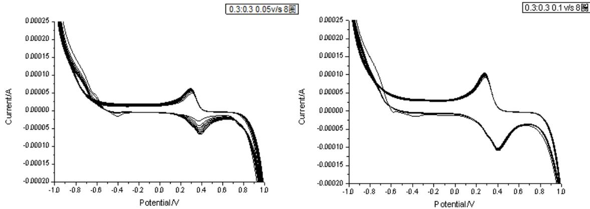
The figure 2-5 the cv curve of PANI prepared in different scan rate when the solute concentration ratio is 0.3:0.3
