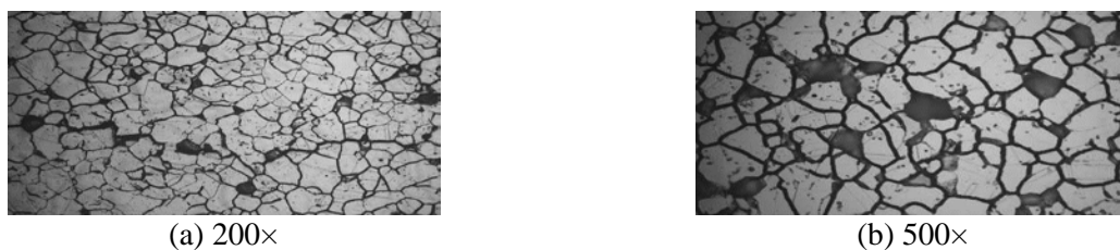
Figure 2. Non-magnetic drill collar metallographic structure
