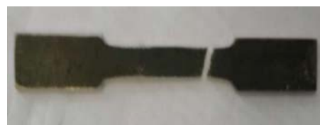
Figure 4. Fracture specimen
