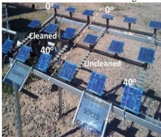
Figure 3. Experimental set-up for studying the effect of tilt angle on soiling [9].
