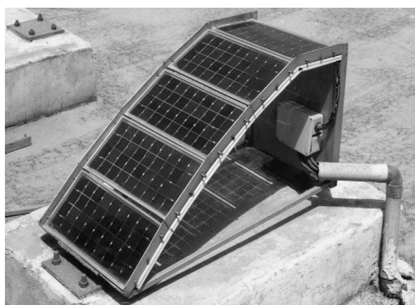
Figure 6. Experimental set-up for studying the effect of tilt angle and air pollution [11].
