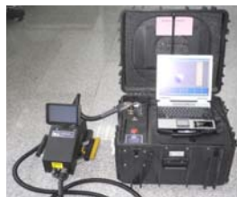
Figure 1. Laser dislocation speckle interference detection device
