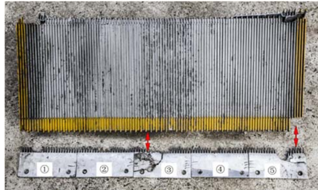
Figure 1. Escalator step and comb plate.
