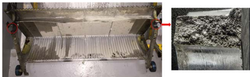
Figure 4. Macroscopic fractography of the escalator step support.
