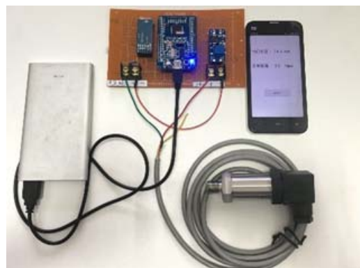
Figure 5. Leak detection system diagram
