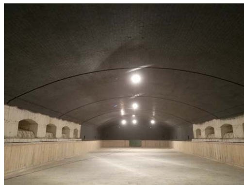
Figure 5. The infrared radiation coating sprayed on the inner surfaces of glass furnace
