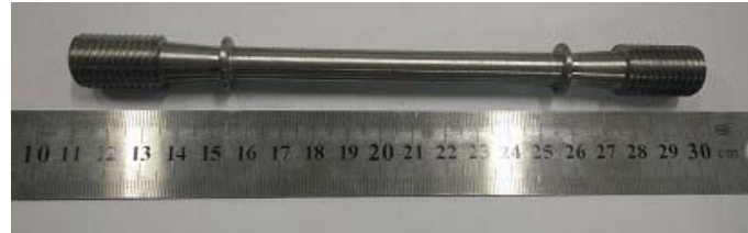
Figure 1. High temperature creep specimen of 10MoWVNb steel
