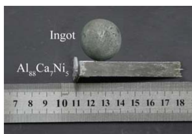
Figure 1. The outer shape and surface appearance of the as-cast wedge sample and ingot of the \text{Al}_{88}\text{Ca}_7\text{Ni}_5 alloy.
