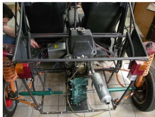
Figure 3. Rear axle with conventional passenger-car final drive, driven by IC engine.
