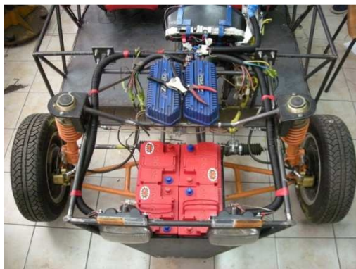
Figure 2. Front axle with in-wheel electric motors and batteries.
