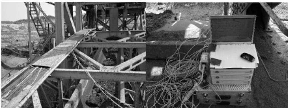
Figure 10. Cabling and tension-metric measurement on the arm of the bucket holder wheel.
