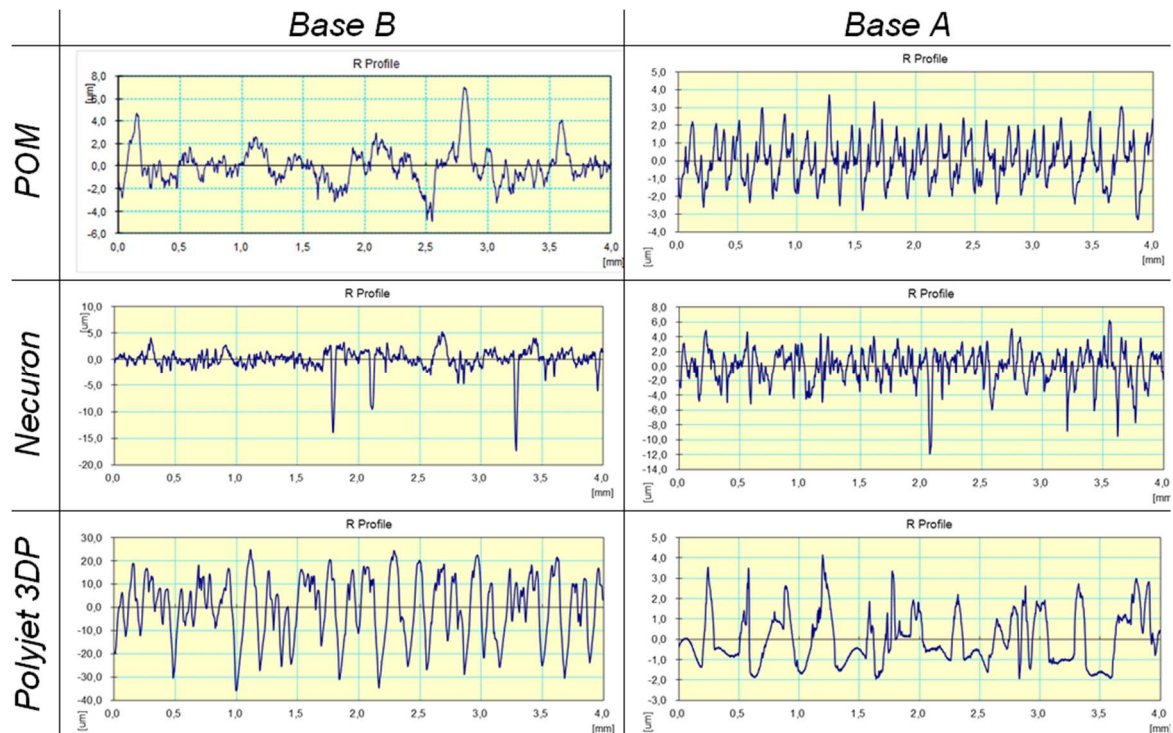
Figure 3. Surface roughness plots of the examined workpieces.
