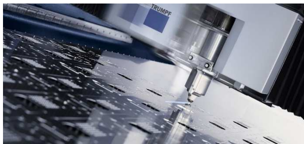
Figure 1. Photo of the laser cutting process.
