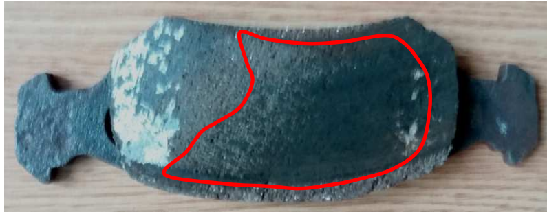
Figure 6. Plate disc contact surface during the experiments.
