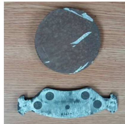
Figure 4. Metal support and the composite material sample.
