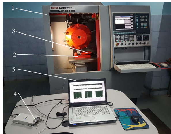
Figure 4. Experimental setup and measuring chain: 1- milling centre, 2- vise, 3- accelerometer, 4- acquisition module, 5- laptop.
