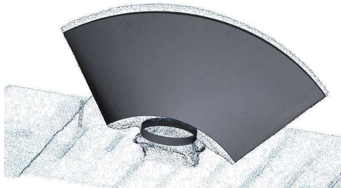
Figure 11. The blade surface and the trunnion cylinder.
