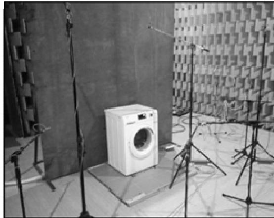
Figure 1. Appliance placed in an acoustic anechoic chamber.
