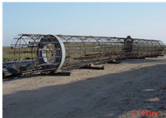
Fig.2 Load box and steel cage in self-balance test
