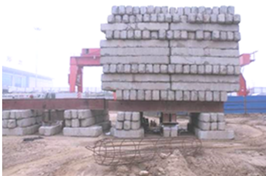
Fig.1 Photo of static load test
