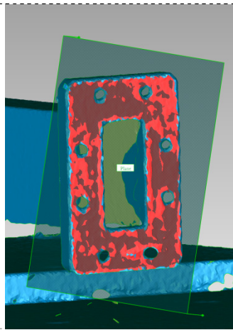
Figure 4. Feature Extraction of docking surface of Waveguide
