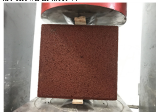
Figure13. Water permeable brick splitting tensile test
