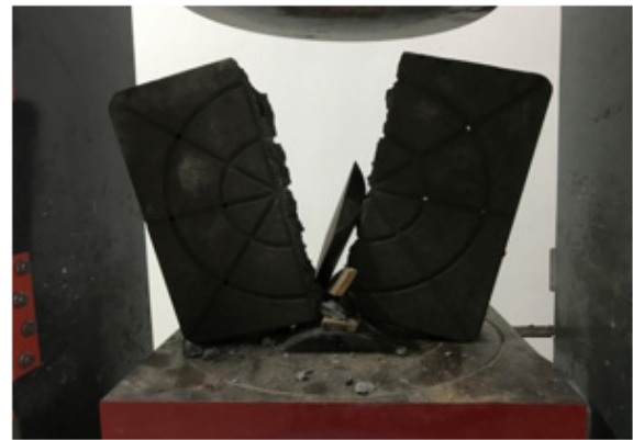
Figure 7. The fracturing tensile test of the brick was destroyed
