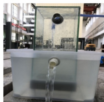
Figure5. Experimental apparatus for water permeability coefficient
