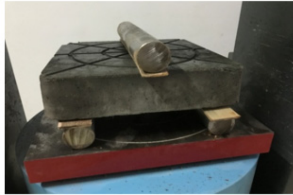
Figure3. Schematic diagram of anti-folding test
