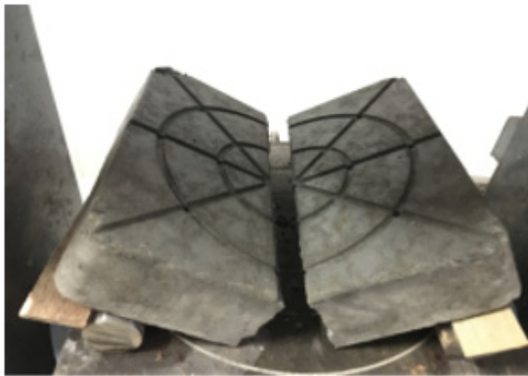
Figure 6. Anti-fold test brick damage graph
