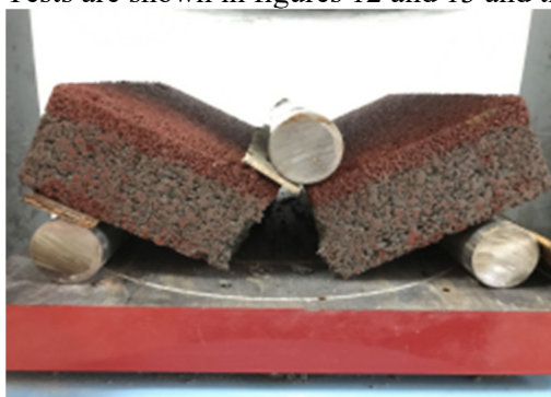
Figure12. Permeable brick flexural test
