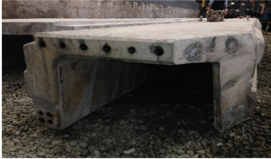
Figure 1 High-strength prestressed concrete grooved sheet pile
