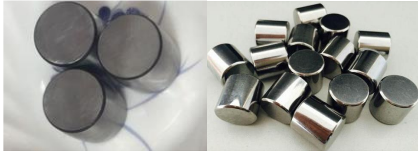
Figure 4. Specimens for impact experiments of P110S under high strain rate and dynamic loads
