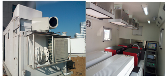
Fig.1 Picture of SO 2 and NO 2 DIAL and its deployment being developed
