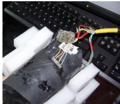
Figure 6 Paste method of strain gauge with ASR test methods
