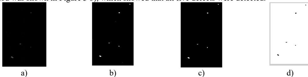
Figure 3. Defect image segmentation and morphological processing, a) Gray scale of defect to be measured, b) Binarization of defect image, c) Morphological processing, d) Image inversion
