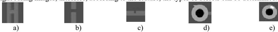
Figure 5. Defect Type, a) Short circuit, b) Open circuit, c) Depression, d) Protrusion, e) Hole
